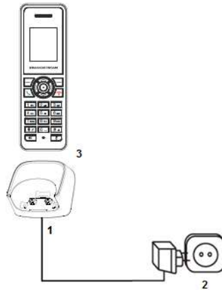
Figure 6: Setting up the charger station
